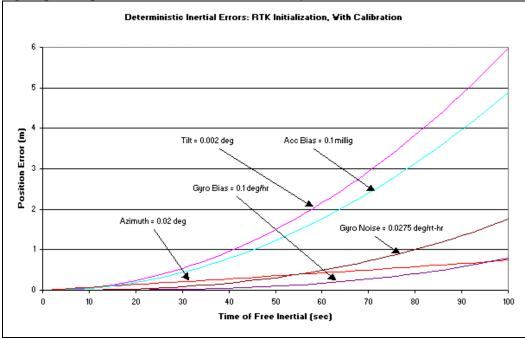
The following Figure 3 shows the combination of all the deterministic position errors in an RMS plot that compares
