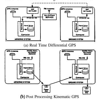
Figure 2. System Configuration
