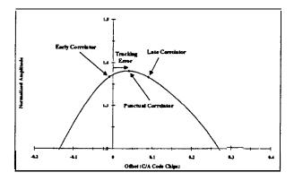
Figure 4: Tracking Error Due to Multipath
