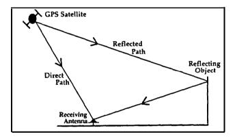
Figure 1: Direct Path and Multipath (Reflected Path) Signals
