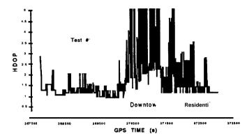
Figure 4: GPS HDOP (Height Fixed) Observed, June 3, 1993, 0000-0130
