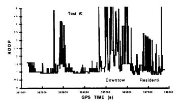
Figure 5:GPS HDOP (Height Fixed) Observed, June 3, 1993, 0630-0830
