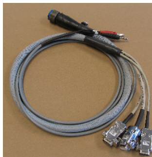
Figure 30: iIMU-FSAS Interface Cable
