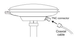
5. Attach the other end of the coaxial cable to the antenna input port of the receiving device, which must provide power as detailed in the *SPECIFICATIONS* section of this guide. All NovAtel GPS receivers provide the necessary power through their antenna RF connectors.
