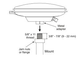
The metal adapter on the bottom of the antenna is fixed in place. Do not attempt to remove it.
