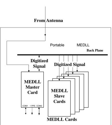
Figure 2 Portable MEDLL Receiver Functional Block Diagram
