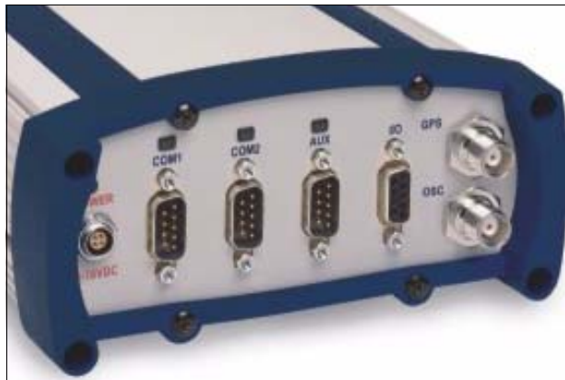
Figure 4: Close-up of Ports on Back End-Cap
