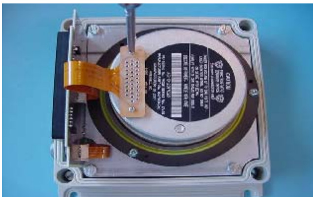
Figure 25: Secure the Connector
