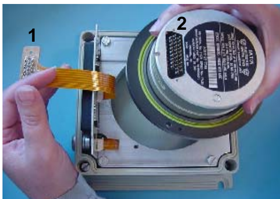
Figure 20: Install the IMU Gyro into the Enclosure Base
