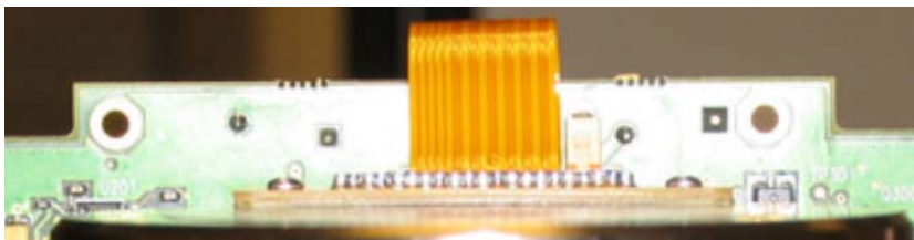
Figure 24: Correct (Flat) Flex Cable Installation
