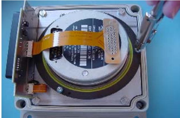
Figure 21: Threadlock and Torque 3 Screws
