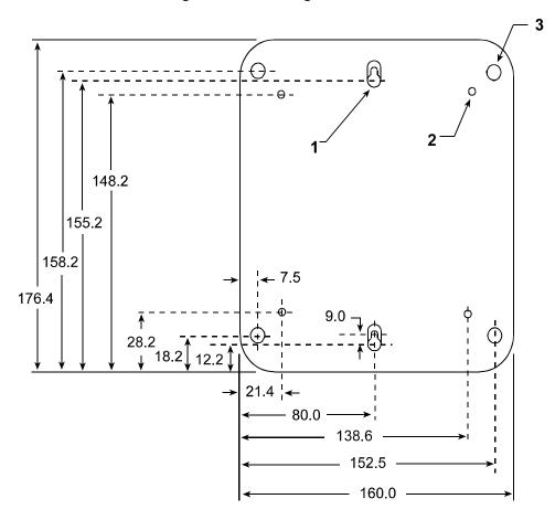
Figure 15: Mounting Bracket Drill Holes - Dimensions
