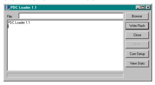
Ensure your PC and DL are properly connected, see *Setting Up At The Office*, *Page 15*. The serial data cable should go from any COM port on the PC to COM2 on the DL. Have all power cables in place but do not turn on the DL just yet. Power the DL using the AC adapter. Do not use batteries, as power interruptions during the process may damage the DL, see the warning below.
