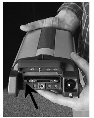
Figure 7: Handling the PC Card
