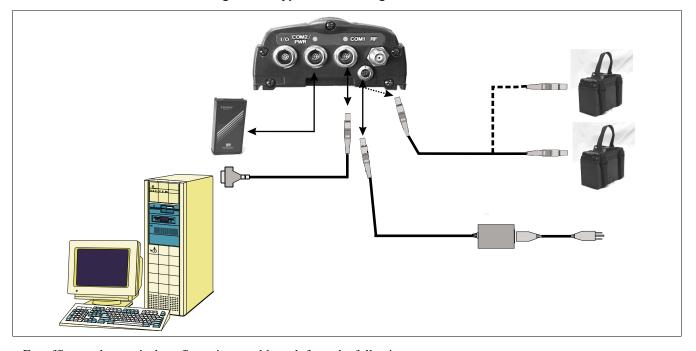
Figure 2: Typical DL Configuration - Office
