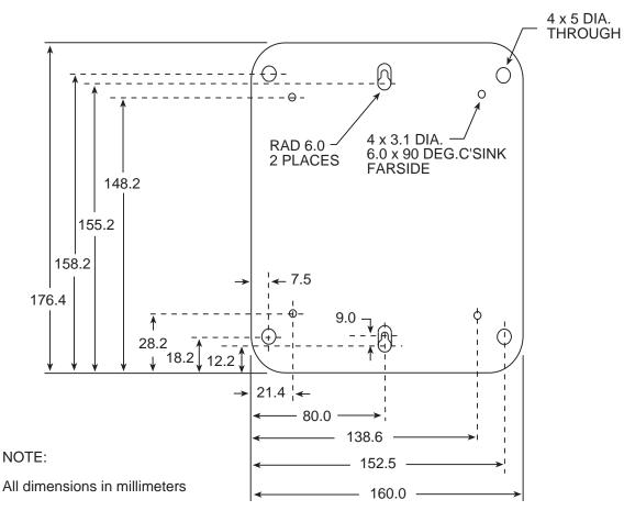
Figure 24 Mounting Bracket Drill Holes – Dimensions
