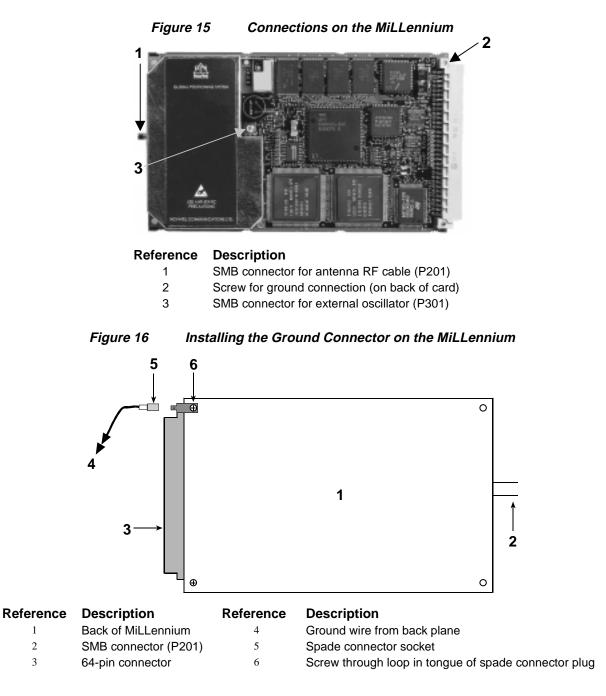
10. The external oscillator interconnect cable is the longer of the two coaxial cables. One end of this cable is attached to the front panel of the PowerPak II enclosure; attach the right-angled SMB connector on the other end to the SMB male jack (P301) on the component side of the MiLLennium (see *Figure 15, Page 48*).
