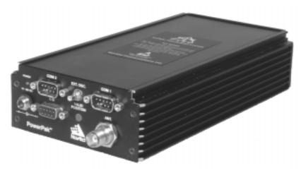
The NovAtel PowerPak II provides a hardware interface between your equipment and the NovAtel MiLLennium GPSCard. When connected to an antenna and a power source, the PowerPak II and MiLLennium together form a fully functioning GPS receiver. This is only one possible application of the PowerPak II; it can also be used by a system integrator to test and evaluate MiLLennium GPSCards.
