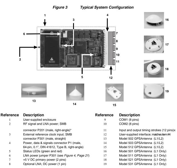
\* To antenna via interconnecting coaxial cable. High quality coaxial cable should be used because a mismatch in impedance, possible with lower quality cable, produces reflections in the cable that increases signal loss.
