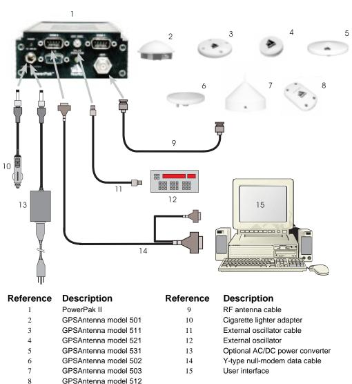
Figure 14 Typical PowerPak II Installation Configuration
