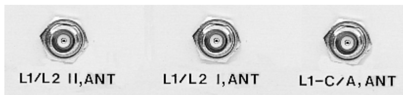
Figure 24 Antenna Input - GUS
