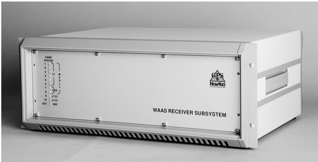
Figure 2 The NovAtel WAAS / GUS Receiver
