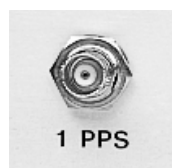
Figure 10 1 PPS Output - WAAS
