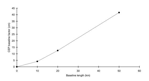
Figure 11-4 CEP Accuracy Degradation with Increasing Baseline
