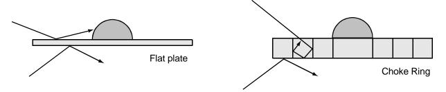
Figure 12-4 Example of GPSAntenna on a Flat Plate vs. Choke Ring Ground Plane
