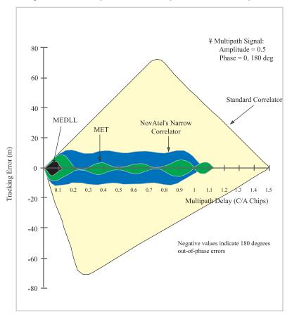
Figure 12-5 Comparison of Multipath Error Envelopes
