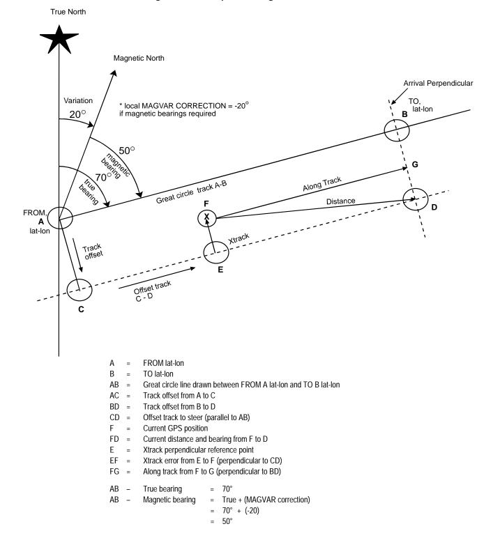
Figure 5-1 Example of Navigation Parameters
