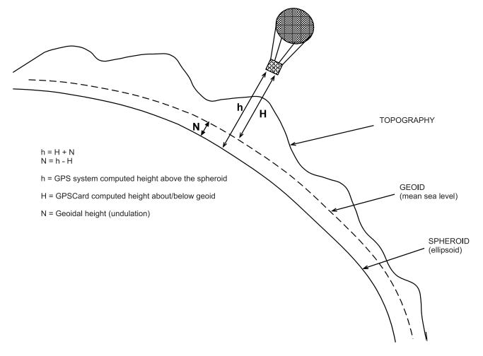
Figure 5-2 Illustration of GPSCard Height Measurements
