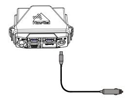
5. Plug in the adapter and/or turn on the power supply. The LED will be red when the FlexPak is properly powered.
