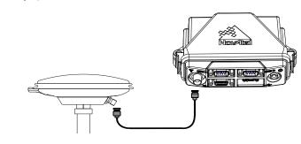
Connect the COM1 or USB port on the receiver to the USB or serial port on the PC. If you are using a USB connection, install the USB drivers available on the CD provided.
