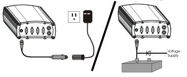
You may also have a user point device such as video equipment. Connect the device to the receiver's I/O port using a cable that is compatible to both the receiver and the device. Refer to your device's documentation for information on its connectors and cables. The arrow along the cable in the figure indicates a MARKIN pulse, refer to *Volume 2* of the *OEM4 User Manual* set, from the user device on the right to the DL4*plus* I/O port.
