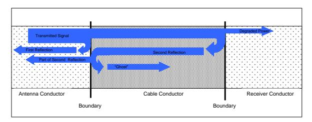
Many times, users will buy "Very Low Loss RG-59" cable because it looks very similar to the RG-58 cable that is supposed to be used. The main difference is that the impedance of RG-59 is 75 ohms and the impedance of RG-58 is 50 ohms. GPS receivers and antennas typically have an impedance of 50 ohms.
