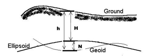
N = geoid / ellipsoid separation or geoid undulation
